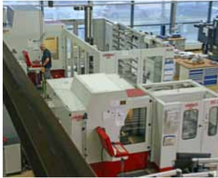
The two automated Röders production cells. In the foreground an RXP 500 DS with RC 2 carousel magazine, partly concealing an RXP 601 DSH with expandable RCM linear magazine for workpieces and tools (Photo: Klaus Vollrath)
