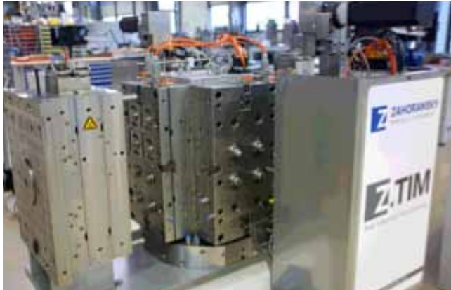
The Z.TIM stack injection moulding tool consists of two tool sides with a central rotating cube. This makes it possible to produce two different parts on one tool (Photo: Klaus Vollrath)
