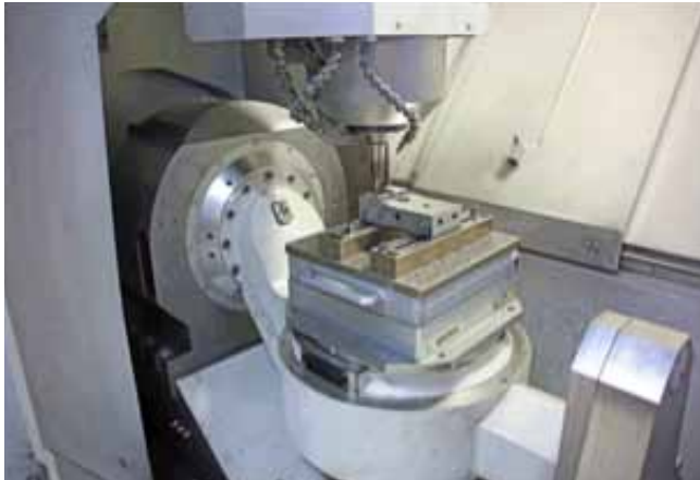
The workspace of the RXP 601 DSH. In the middle is the robust tilting rotary table, supported on both sides. The counter bearing on the right side has a loading capacity of 7,000 kg (Photo: Klaus Vollrath)
