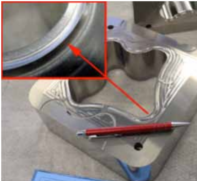
Massive fine stamping matrix made from ultrahard tool steel. Typical features include the fine-ground vertical inner and outer contours as well as the v-shaped protrusion closely following the contours of the part (Photo: Klaus Vollrath)
