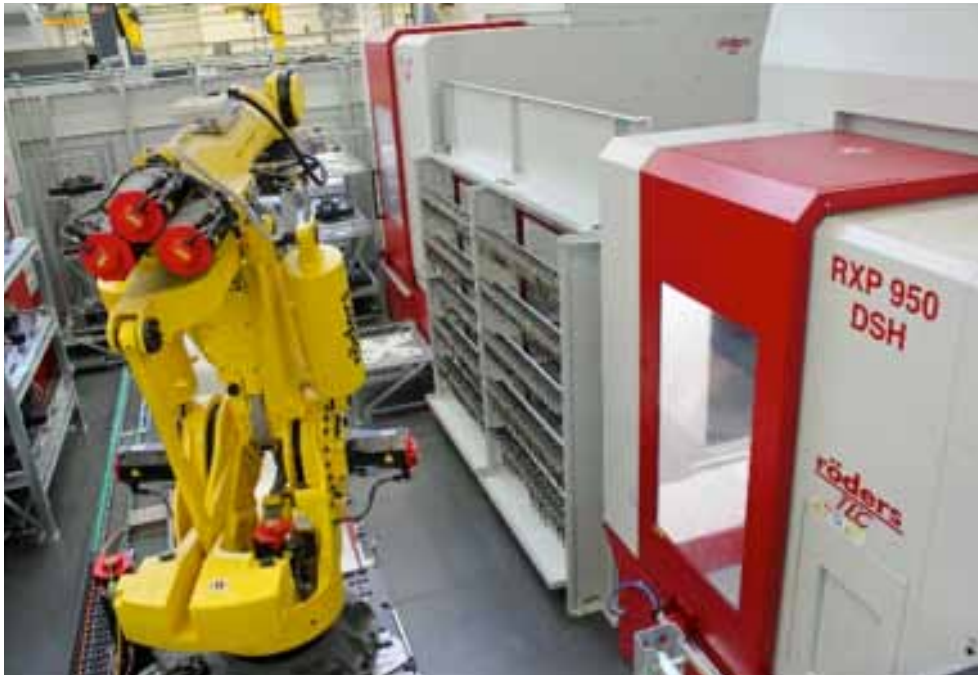
Current status of the fully automated production cell with two RXU 1200 DSH milling centres, one RXP 950 DSH system and a robot with a gross carrying capacity of 790 kg and a large store for cutting tools and pallets (photo: Klaus Vollrath)
