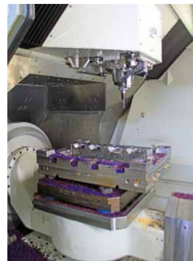
Noticeable features in the working space are the robust z-axis, which is particularly rigid due to the guides on all four corners, and the stable rotating/swivelling table, which is supported by bearings on two sides (photo: Klaus Vollrath)
