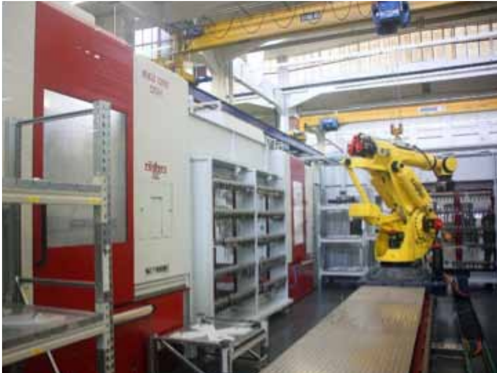
Since being extended, the cell has had a total of 543 internal and external tool positions as well as 21 pallet spaces for workpieces (photo: Klaus Vollrath)
