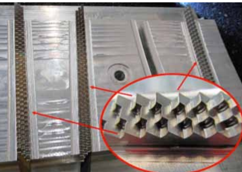
Irrespective of their robustness, the plants are even sufficiently precise to be able to machine very fine details with milling cutters down to diameters of 0.4 mm (photo: Klaus Vollrath)
