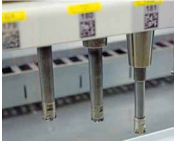
The spindles with cutter heads of up to 35 mm in diameter machine the material with a hardness of up to 50 HRC (photo: Klaus Vollrath)
