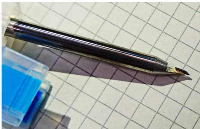
Milling tool with diamond tip for machining non-ferrous metals on the Röders milling machine (Photo: Klaus Vollrath)
