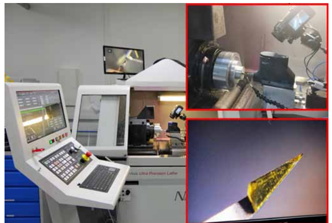
The original business model of son-x was the development of tool holders for ultra-precision turning using diamond tools. The holders vibrate in the range of ultrasonic frequencies (Photo: Klaus Vollrath / son-x)
