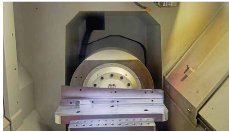
View into the working area of the RXP 601 DSH. Clamped onto the rotary swivel table is a mold insert for light guides, such as those used in automotive interiors (Photo: Klaus Vollrath)
