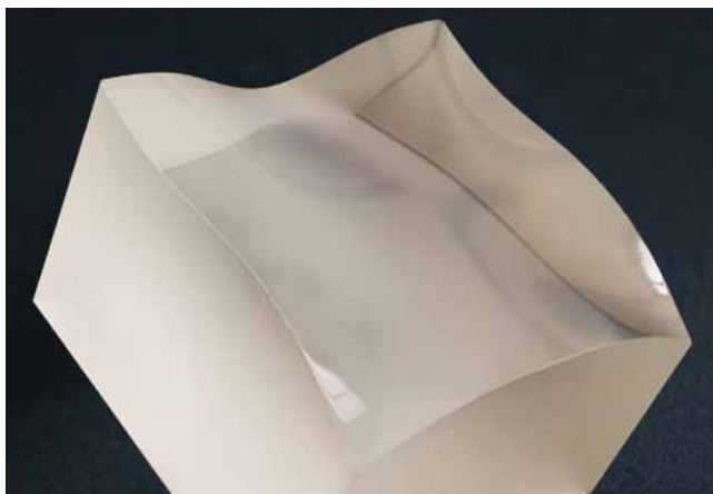
The polished free-form surface on this glass block was produced on a 5axis RXP501 DS milling machine from Röders using grinding points (Photo: ShapeFab)
