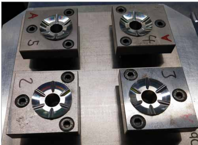
In the setting-up area, workpieces are clamped onto pallets (Photo: Klaus Vollrath)
