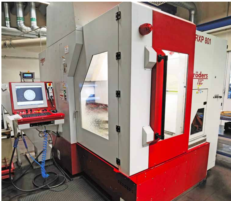
In other shops of the Tech-Centre in Schweinfurt, three-axis Röders machining centres are used for jig grinding (Photo: Klaus Vollrath)
