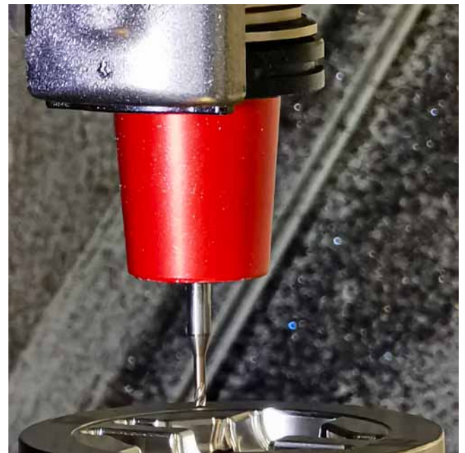
During hard machining, lubrication is supplied through the MHT medium dispenser (Photo: Klaus Vollrath)
