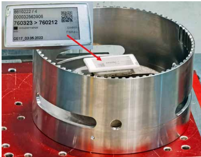
A special tool clamped onto a pallet in the workpiece buffer of the hard machining line. The smart tag programmable by radio frequency holds the key to all process-relevant information, rendering paperwork obsolete (Photo: Klaus Vollrath)
