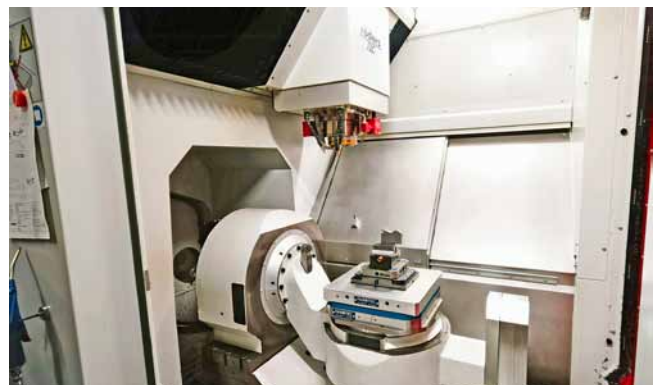
View of the interior: The weight-compensated Z-axis features a length-compensated spindle and alignable coolant spray nozzles. The rotary swivel table is equipped with a zero-point clamping system (Photo: Klaus Vollrath)
