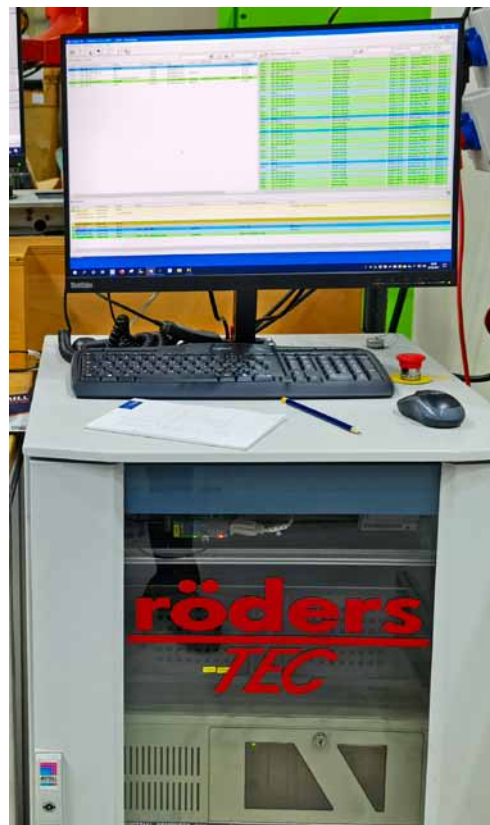
The RMSMain job manager coordinates all processes in the cell and communicates with the work preparation department and Festool's ERP system (Photo: Klaus Vollrath)
