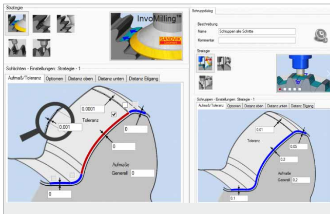
Euklid GearCAM helps users to produce high-precision gearwheels on standard milling machines (Graphic: Euklid)
