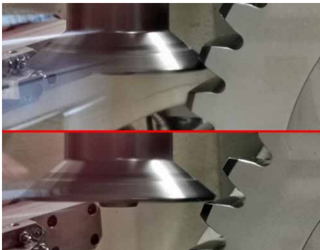
The bevelled shape of the machining tool enables work to be performed on both the left-hand and right-hand tooth flanks without any need to change sides (Photo: Klaus Vollrath)
