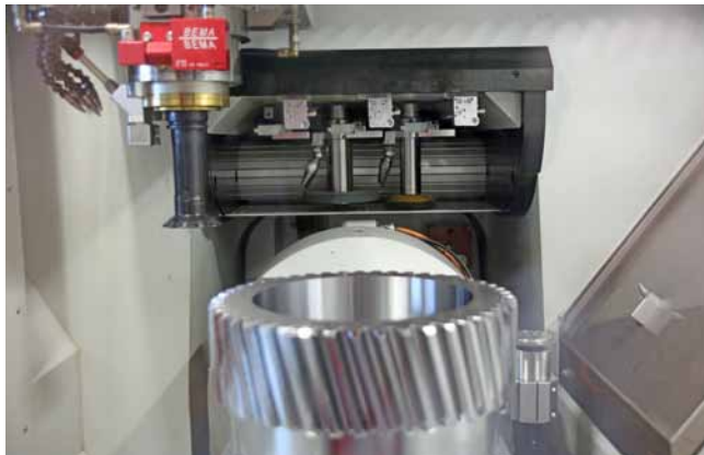
The large-format tools for gearwheel manufacture are stored in a separate magazine below the portal (Photo: Klaus Vollrath)
