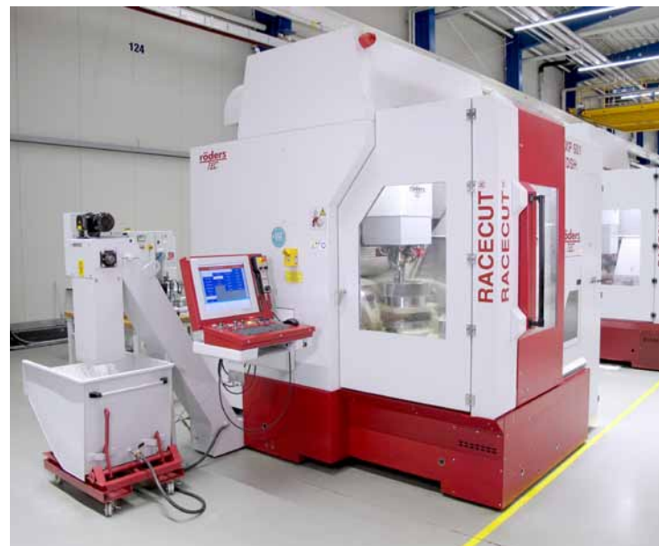
The RXP 601 DSH used as pilot plant for gearwheel machining (Photo: Röders)
