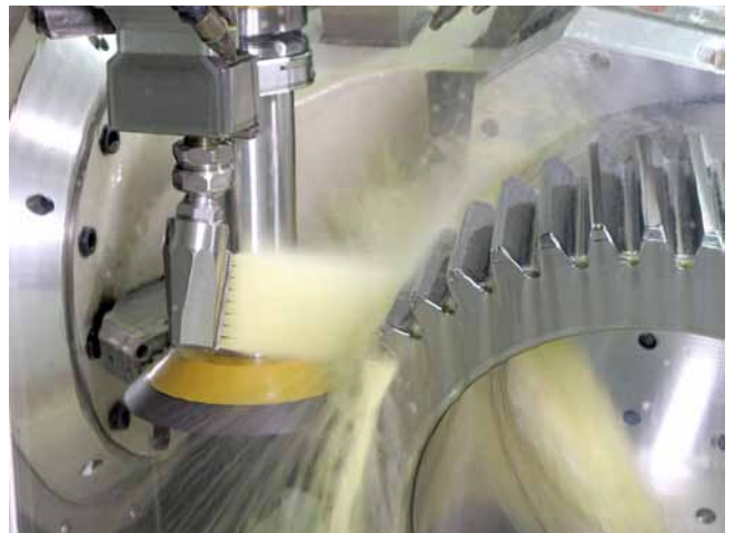
Conical grinding wheel for precise finishing of the tooth flanks (Photo: Röders)
