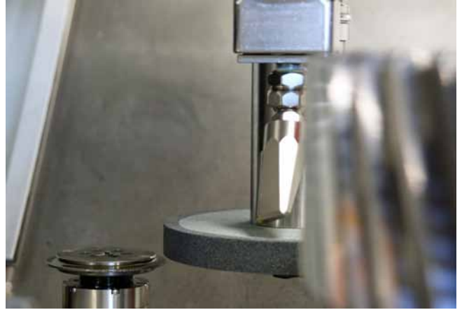
A diamond-coated truing wheel ensures precise shaping of the grinding tools (Photo: Klaus Vollrath)
