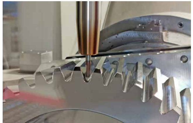
Standard milling cutters from the internal tool magazine are used to produce the tooth root relief (Photo: Klaus Vollrath)
