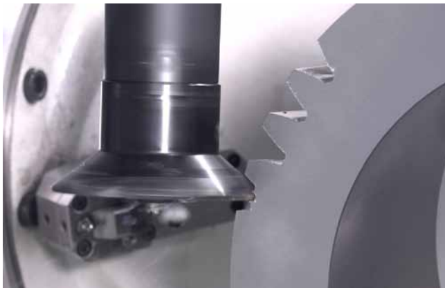
Roughing of the tooth contours in the hardened sprocket is carried out with a conical InvoMilling disc cutter (Photo: Röders)
