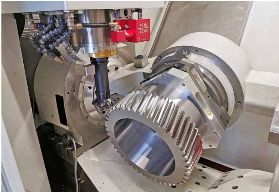
High-quality gearwheels are produced from hardened blanks within a very short time on 5-axis milling centres supplied by Röders (Photo: Klaus Vollrath)
