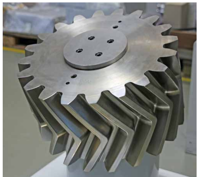
This herringbone spur gear with a diameter of 450 mm and a tooth face width of 250 mm made of 16MnCr5 with a hardness of 60-62 HRC was ready for immediate use after being milled on a Röders RXU 1001 DSH in just 18 h and 45 min (Photo: Klaus Vollrath)
