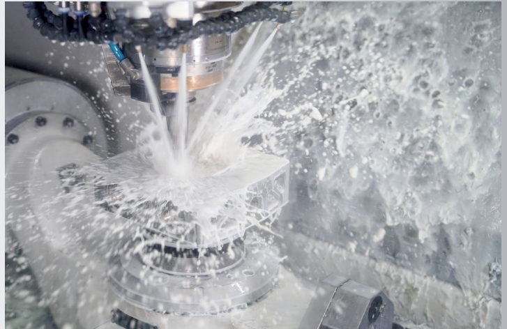
Temperature-stable machining area during machining with emulsion
