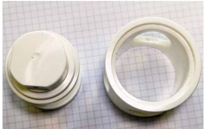
The rotor and housing for handling cryogenic liquefied gases must be machined with µm precision. (Photo: Klaus Vollrath)
