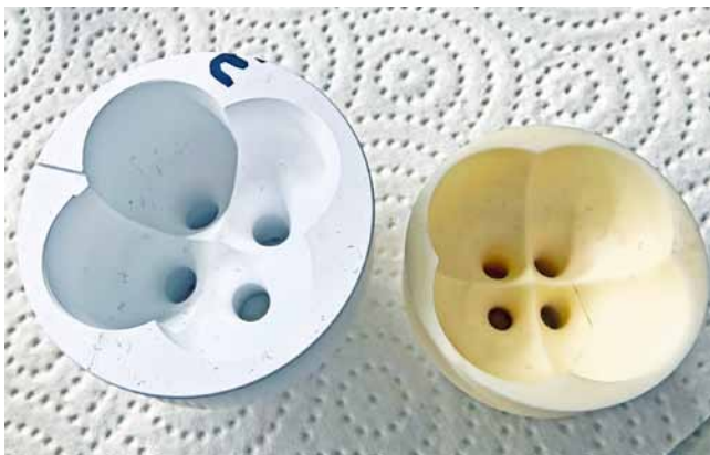
During the sintering process, the component shrinks by around 20 % in all dimensions. This must be taken into account beforehand as an allowance. (Photo: Klaus Vollrath)
