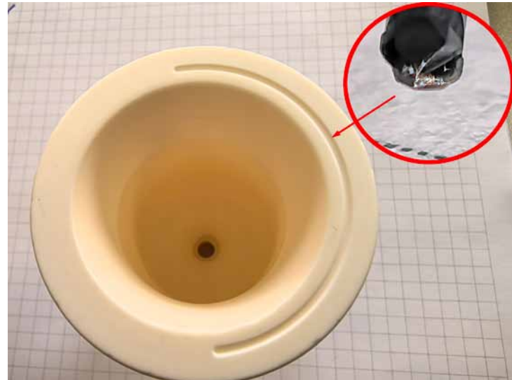
The Zecha ball nose end mill made of diamond-coated solid carbide produced a semi-circular groove 1.5 mm wide and 0.5 mm deep in the upper area of the sintered \text{Al}_2\text{O}_3 ceramic (Photo: Klaus Vollrath)
