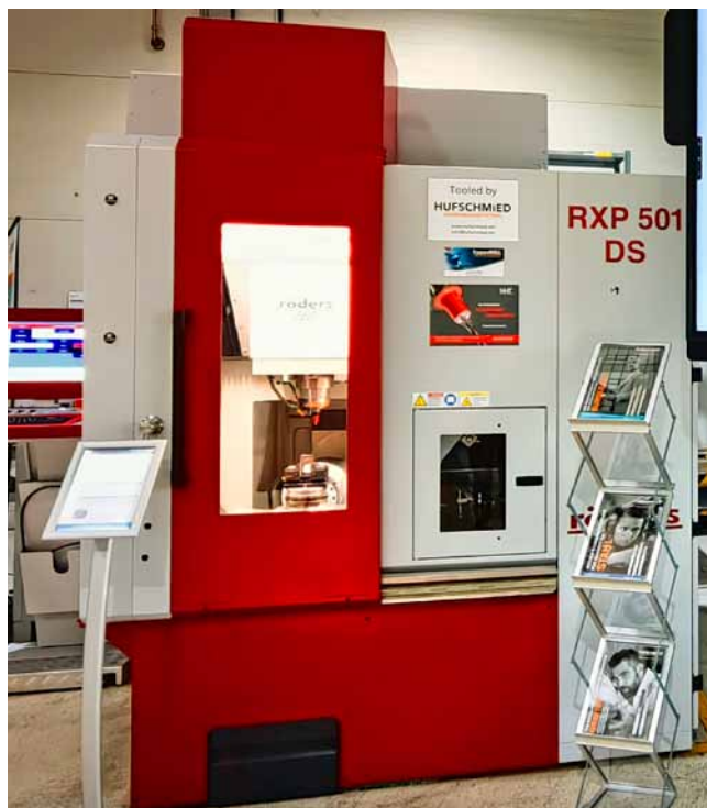
The sample was milled in Hufschmied's technical centre on this five-axis Röders RXP 501 DS. The system is equipped with the MHT medium distributor (Photo: Klaus Vollrath)
