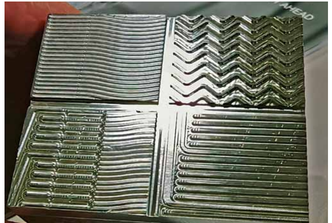
Sample workpiece (50mm x 40mm) with various surface structures typical of bipolar plates made of the Böhler material K888 Matrix with 63+1 HRC (Photo: Klaus Vollrath)
